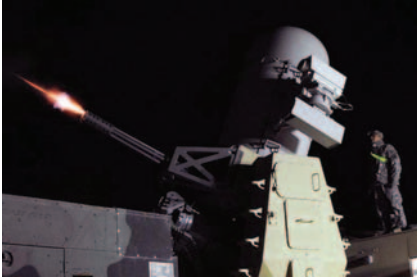
The Counter-Rocket, Artillery, and Mortar (C-RAM) gun can fire thousands of rounds per minute at incoming projectiles.
