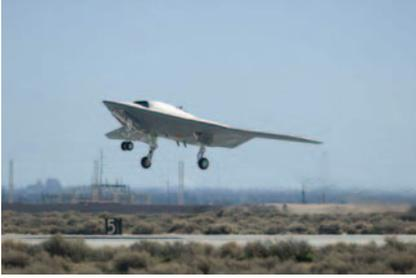
The X-47B unmanned combat aircraft during a 2011 test.
